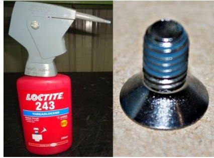
Fig. 1.4.1 Apply enough Loctite 243 to evenly coat the threads of the screws
